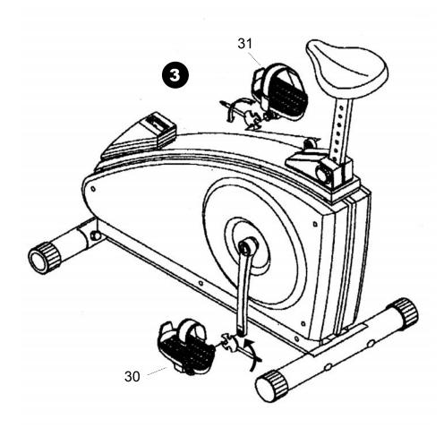
**3.** Attach pedals (30, 31). Axles of pedals are branded "L" and "R." The pedal marked "R" goes on the right hand side of the bike and the one marked "L" on the left hand side. Tighten the left pedal by turning counter-clockwise and the right pedal by turning clockwise.
